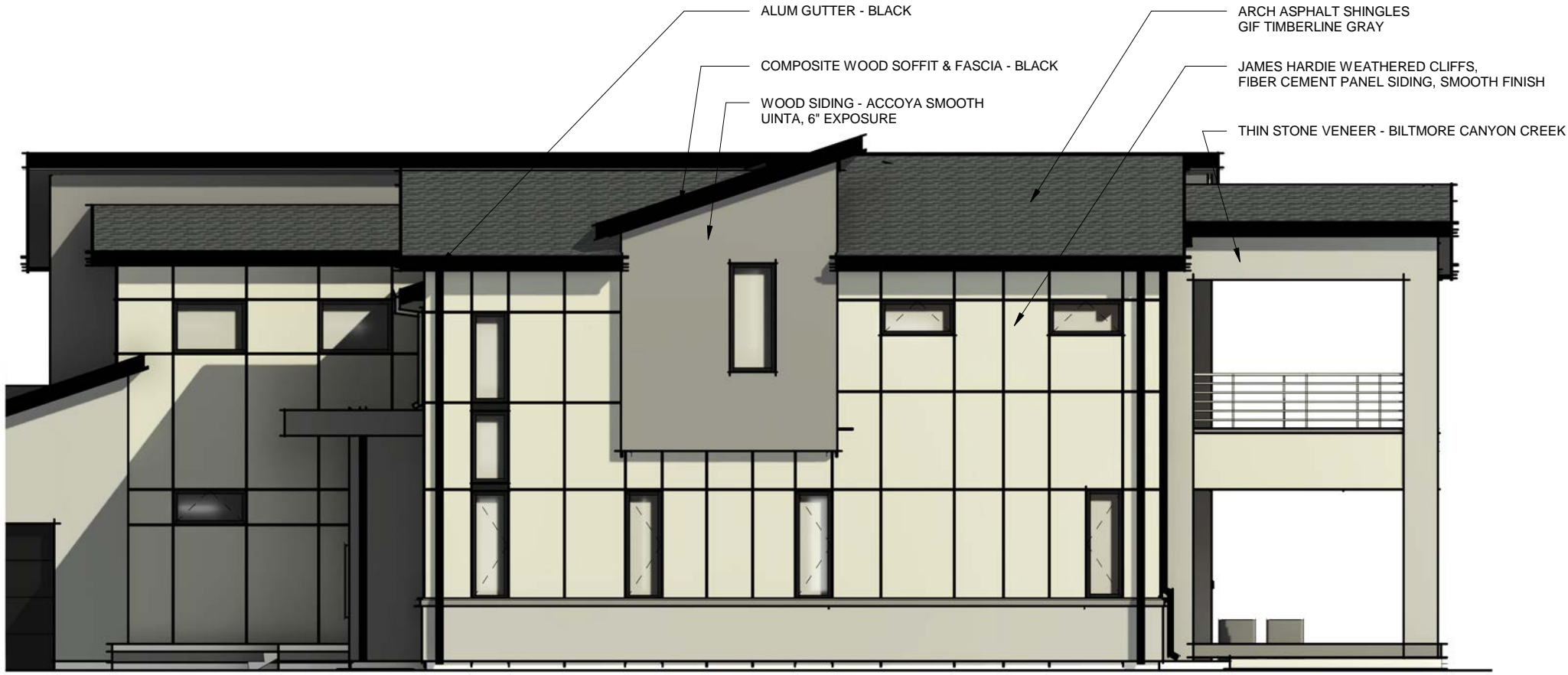
① EAST ELEVATION - HOUSE 1/8" = 1'-0"
