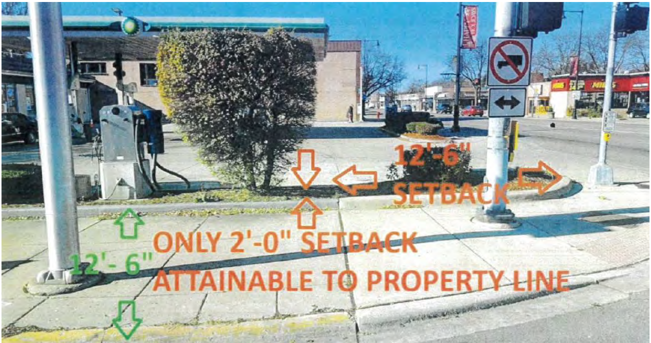
Proposed Pylon Sign Setback Diagram showing Existing Landscaping
