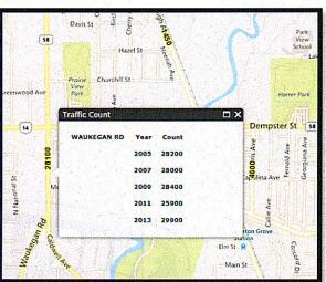
The above maps show the historical Average Daily Vehicle (ADV) counts (traffic volume) for the intersection of Waukegan/Dempster. (*The low volume of traffic in 2011 was most likely due to significant road construction.*)
